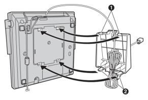
3 Connect the telephone line cord. Mount the base unit by inserting the mounting pins into the round openings on the adaptor (for pin (B), use round cut out at the bottom of the adaptor if you're using the 4 inches phone plate), then sliding the base unit down to secure it.
